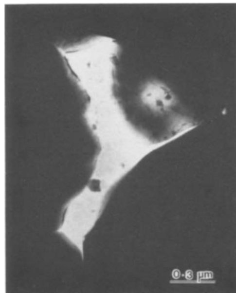
Figure 2 A region of glassy phase, containing a micrograin, situated at a triple junction in the ceramic. BF micrograph.
